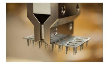
The magnet does not change its magnetic state in case of loss of compressed air.
